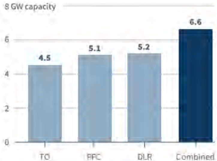
Capacity of queued generation (in GW) enabled to interconnect by each GET, as well as GETs in combination
