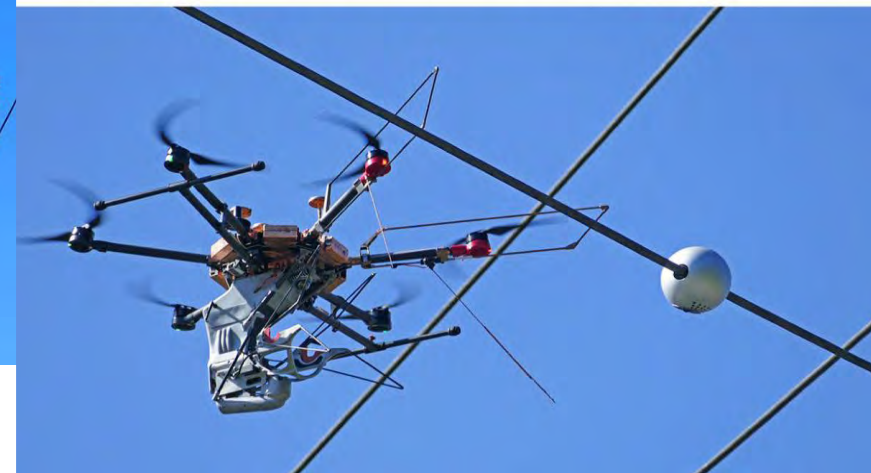
A drone carries the Neuron sensor to a transmission line ( top ). After installing the sensor on the line, the drone flies away ( bottom ).
