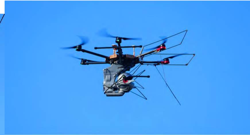
A drone carries the Neuron sensor to a transmission line ( top ). After installing the sensor on the line, the drone flies away ( bottom ).
