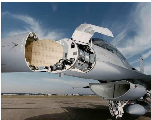
Antenna array of an APG-80 radar installed on an F-16 Fighting Falcon.
